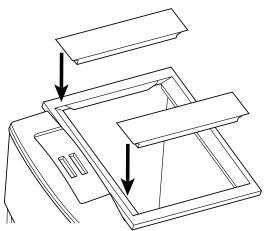
3. Install any necessary Horizontal Filler Plates to top of Vertical Filler Plates in order to fit the unique connection between the icemaker and the dispenser.
